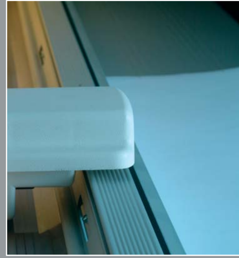
Reversing device for rear delivery of sheets.
